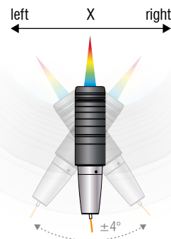
3 Max. tilt angle in X \pm 4^\circ
